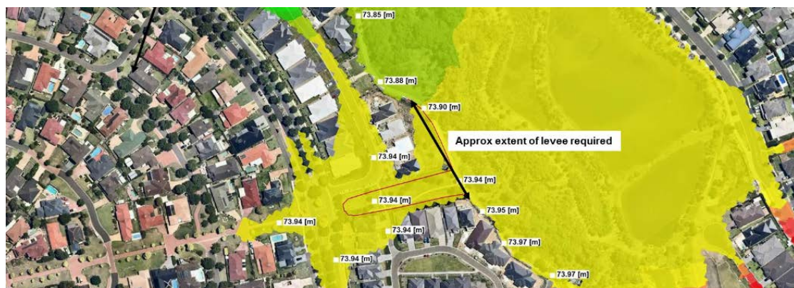
Figure 5-1: Flood Levee Option concept schematic
