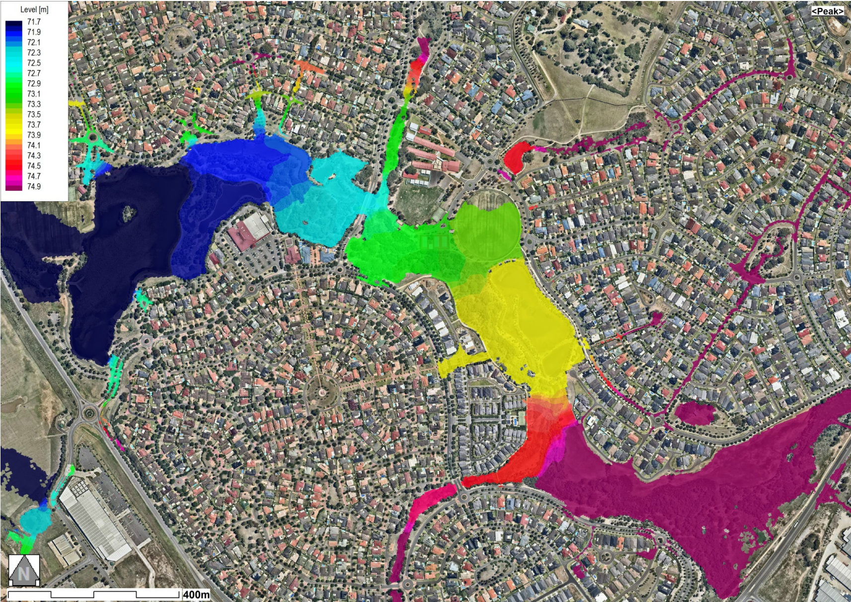
Figure 4-4: Peak 1% AEP flood levels for the Channel Option at Harrington Park
