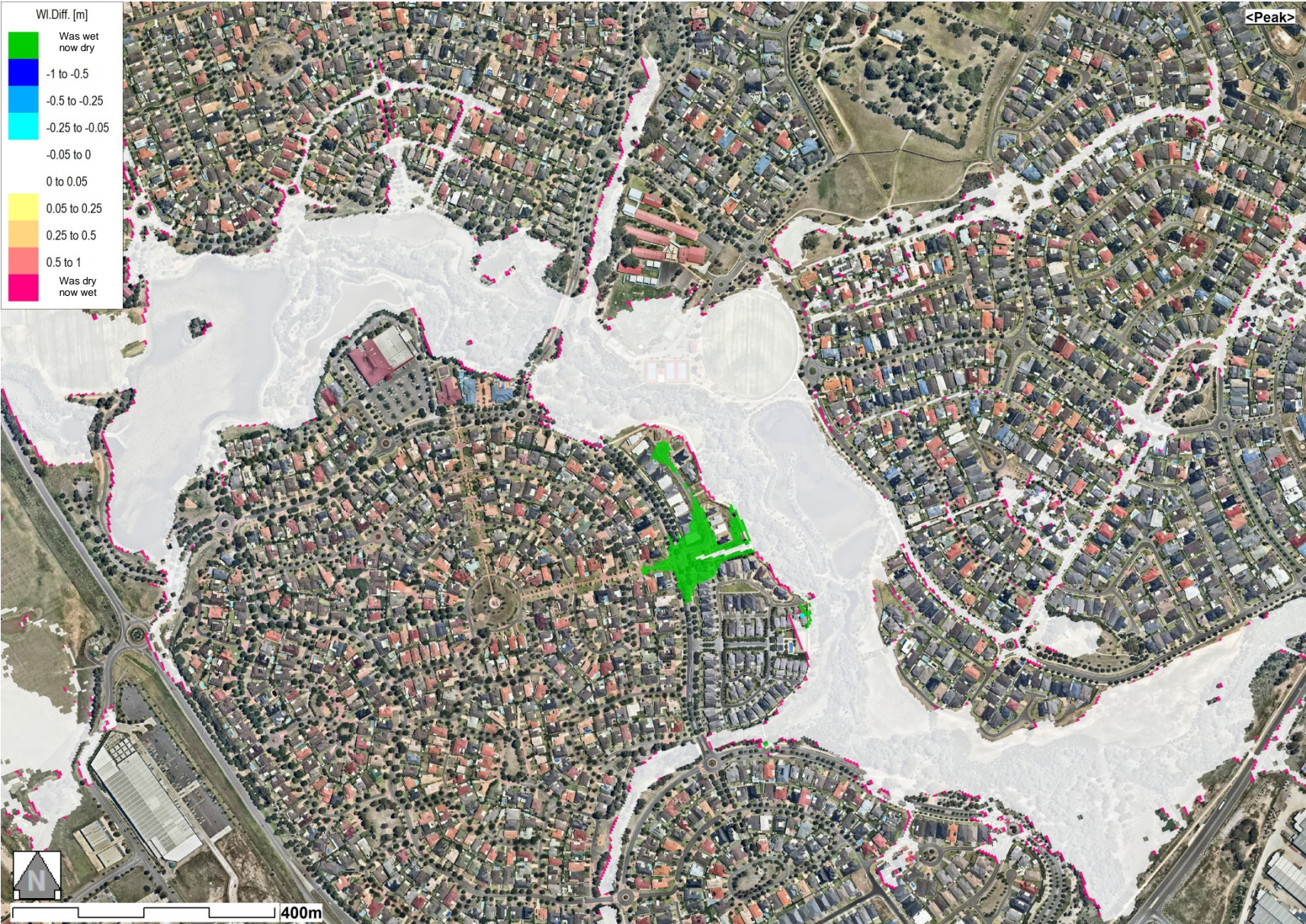
Figure 4-5: Changes in peak 1% AEP flood levels for the Levee Option at Harrington Park
