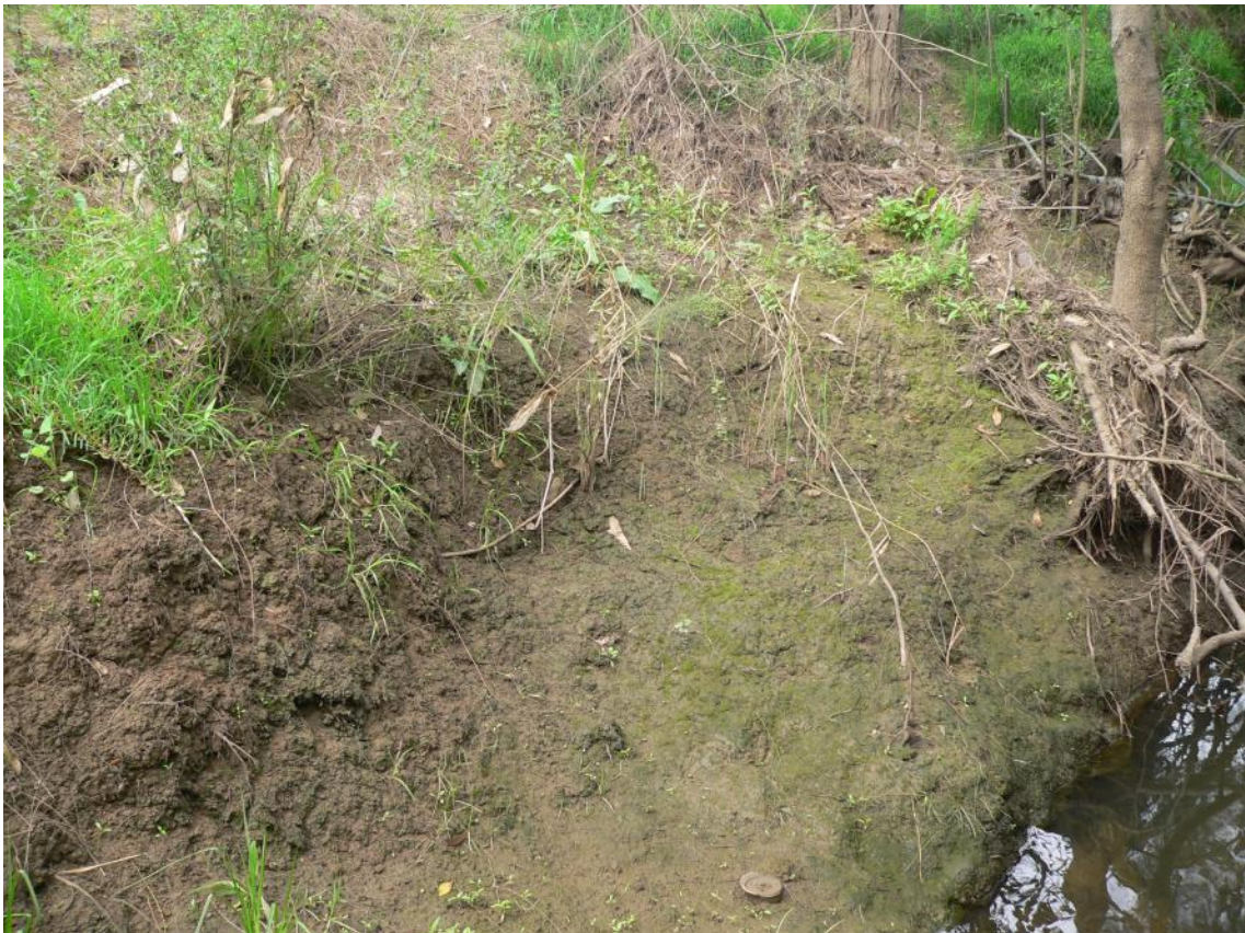
Plate 6: Levee Option 1 - Close up view of slightly sandy clayey silt/silty clay at the toe of the creek's bank.
