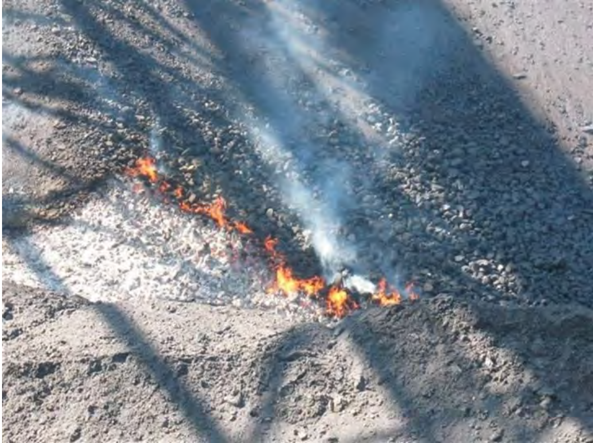
Figure 3. Coal heating developed in uncompact stockpile with steep sides (angle of repose) and coarse coal fraction accumulated at the base of the stockpile allowing pathways for air to enter the stockpile and create a chimney effect. The hotspot has migrated from inside the stockpile to daylight on the surface and reach ignition.
