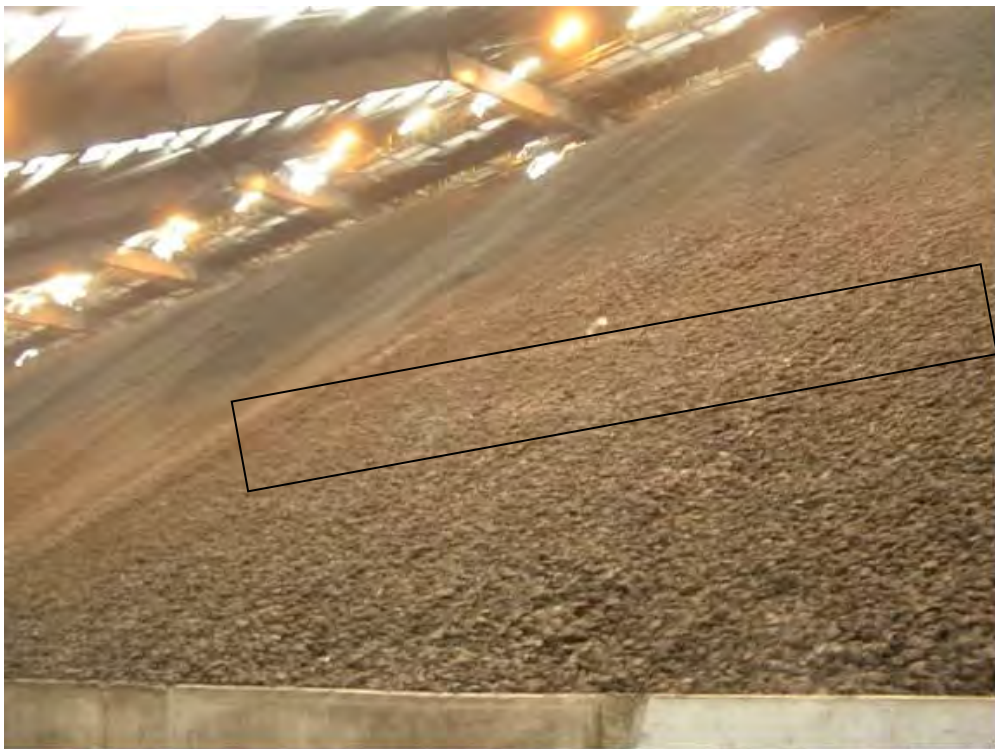
Figure 2. Enclosed stockpile storage of Kideco coal showing no compaction except from the weight of the stockpile and steep sides at angle of repose with coarse coal fraction accumulated at the base of the stockpile allowing pathways for air to enter the stockpile and create a chimney effect. Note the moisture condensation lines within the rectangular zone arising from hot spot development inside the pile. Thermal runaway reached in 10-15 days.
