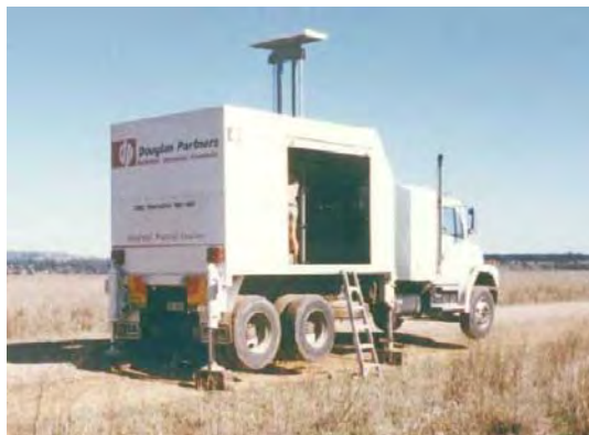
Figure 2: Purpose built CPT rig
