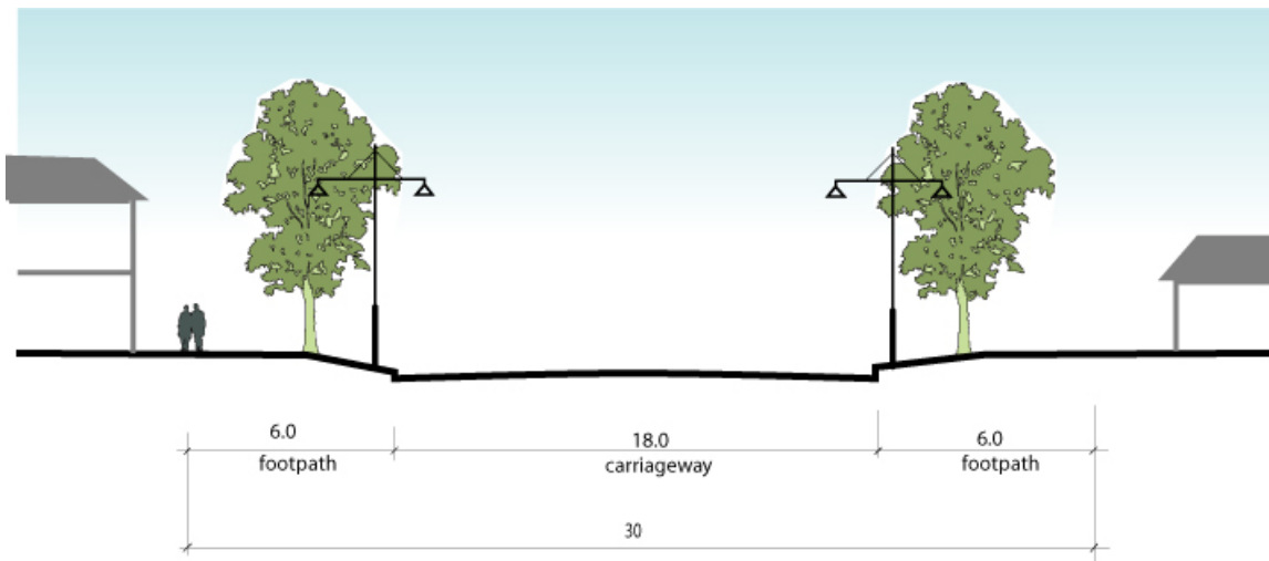
Figure 17: John Street – Section
