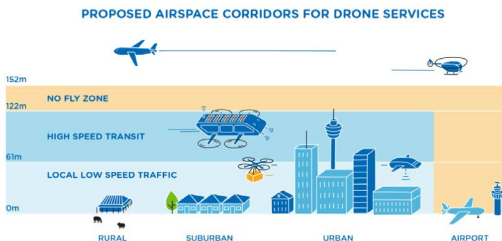
Figure 30 Inspired by Amazon's proposal for segregated airspace below 500ft for the operation of drones ( Forbes Magazine, July 2015 )
