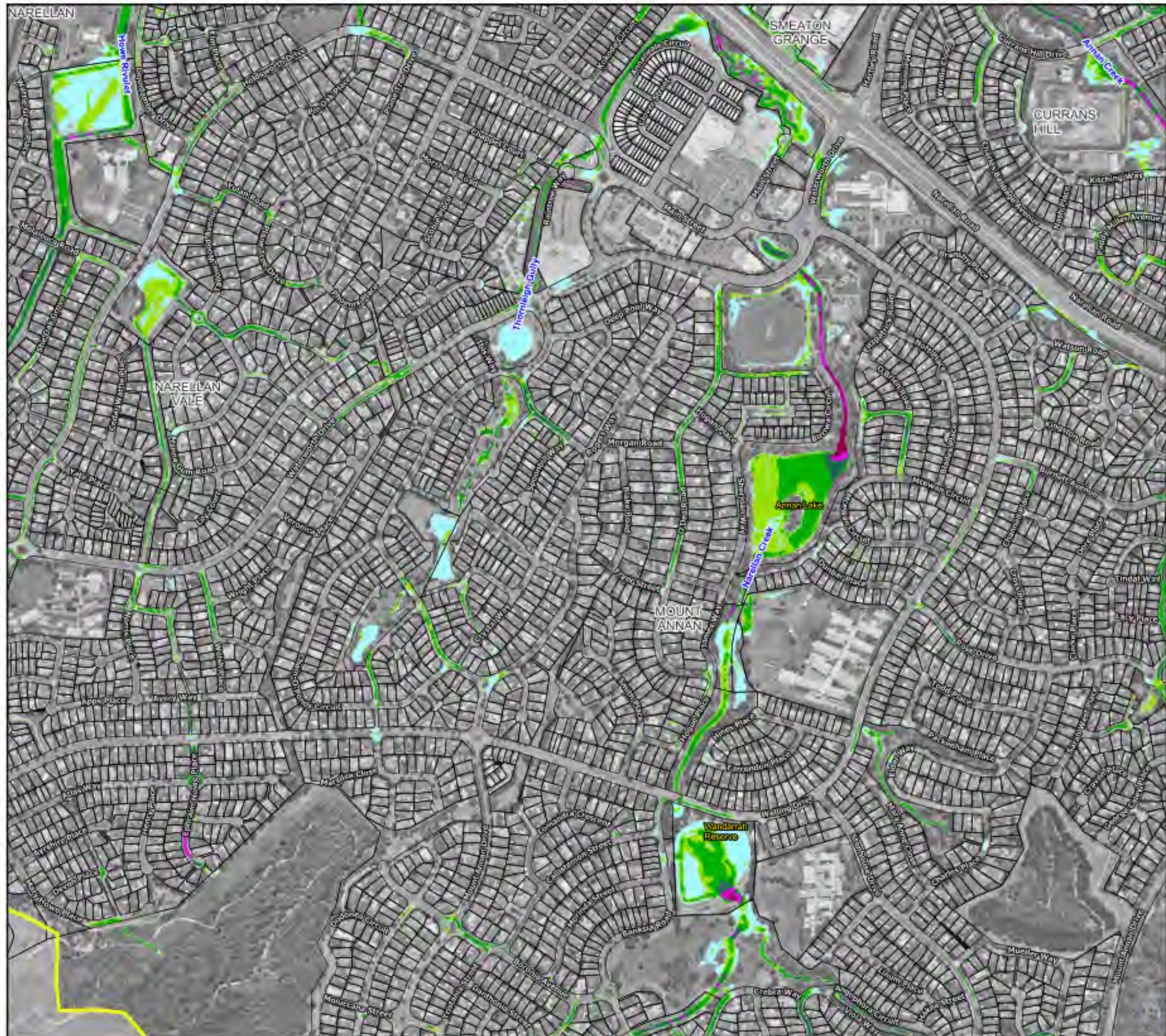
Figure 33.9 : Peak Water Velocities for the 20% AEP Flood
