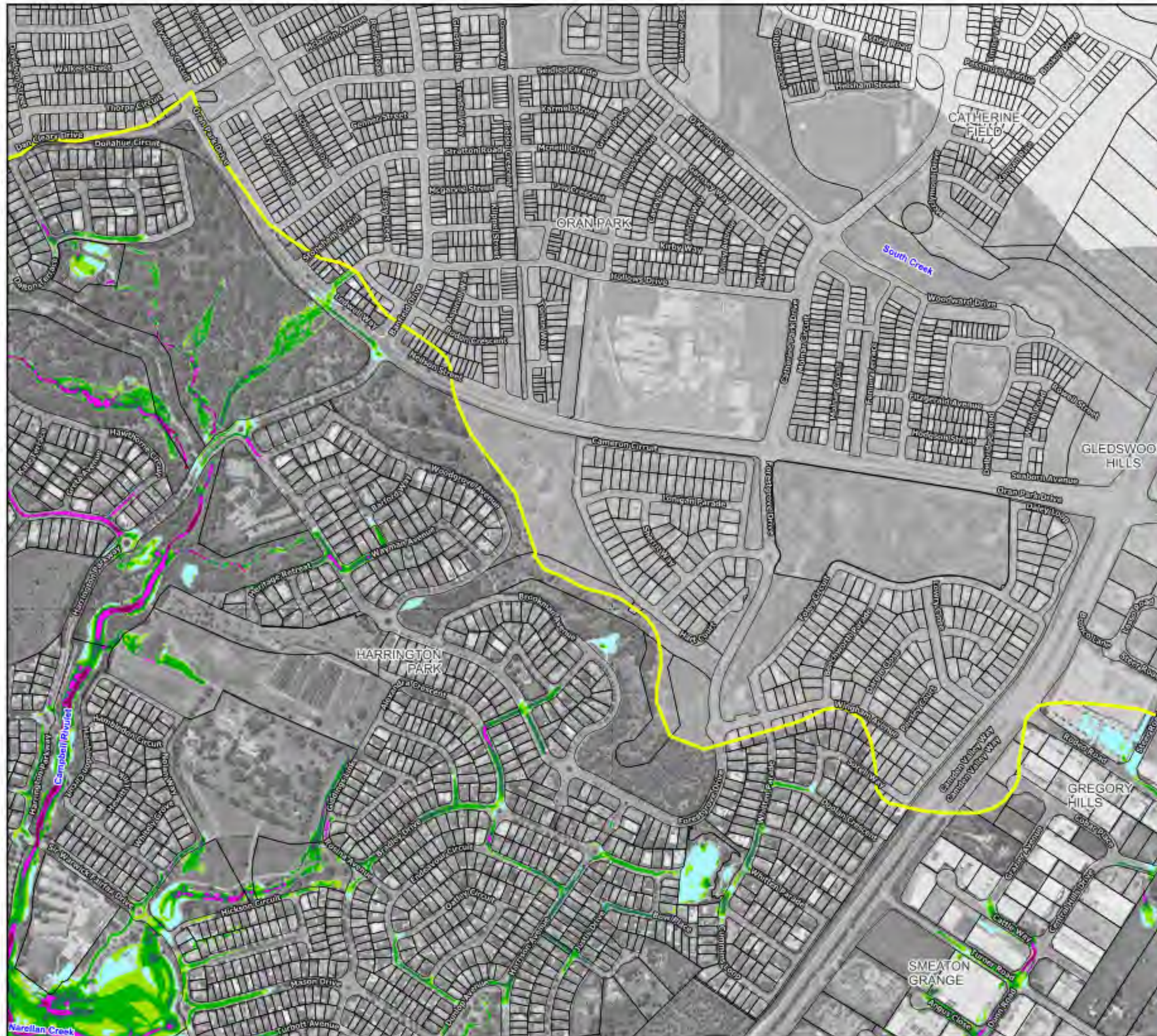
Figure 38.2 : Peak Water Velocities for the 0.5% AEP Flood
