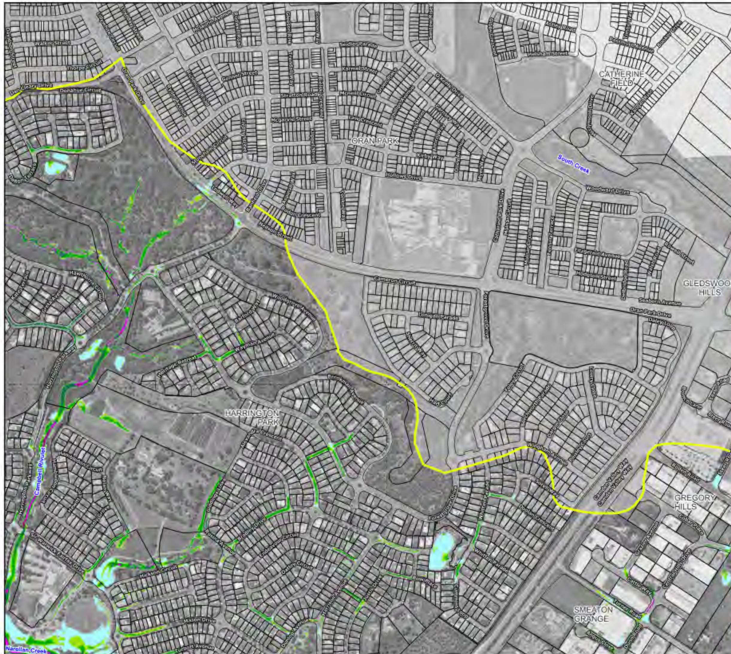
Figure 33.2 : Peak Water Velocities for the 20% AEP Flood
