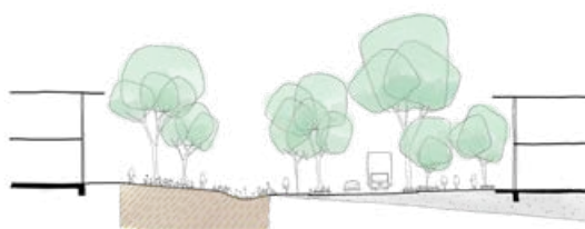
Figure 36: Example of a street cross-section with an offset carriageway to retain a continuous soil corridor.
