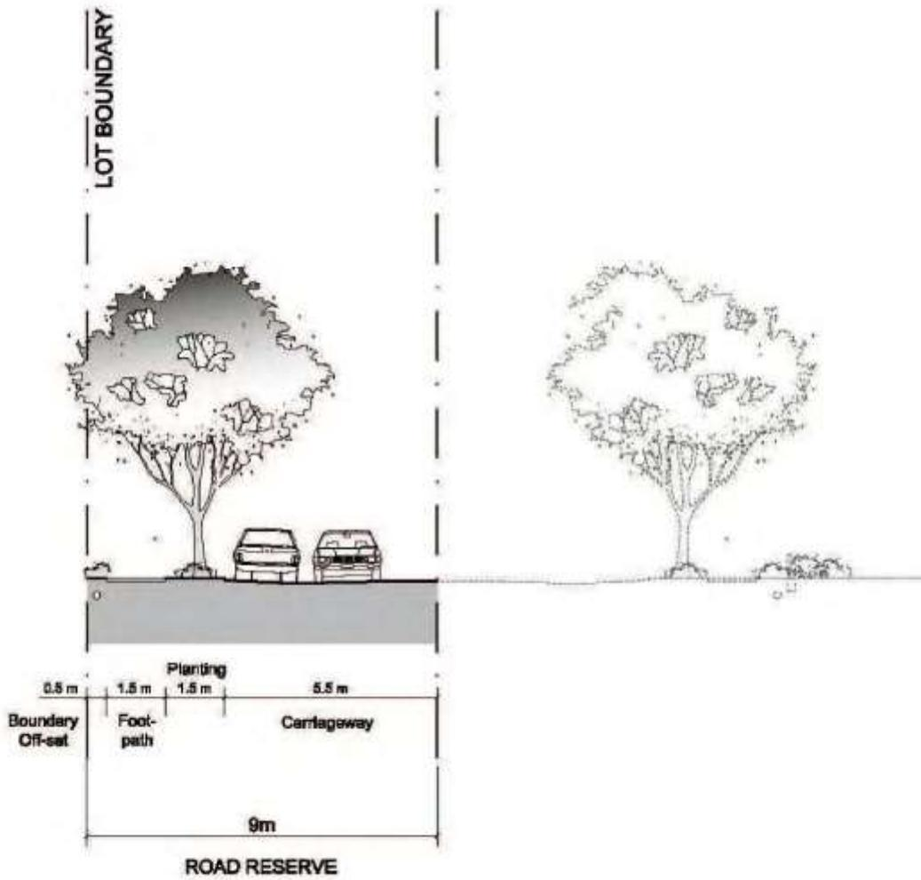
Figure 3-20 Temporary half road width construction
