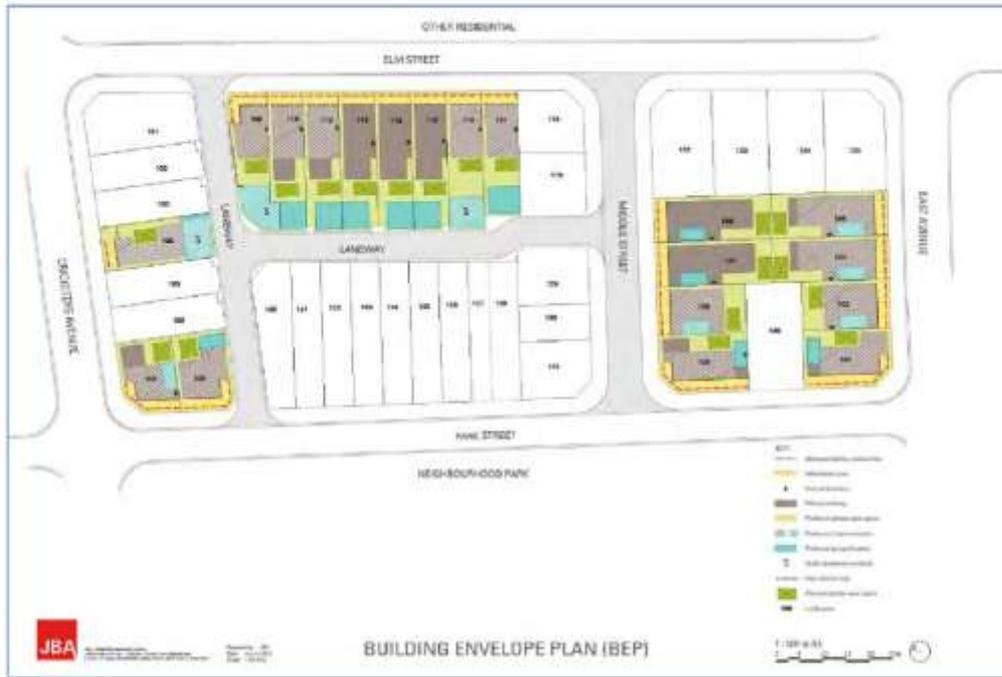
Figure 3-8: Sample of a Building Envelope Plan (BEP)
