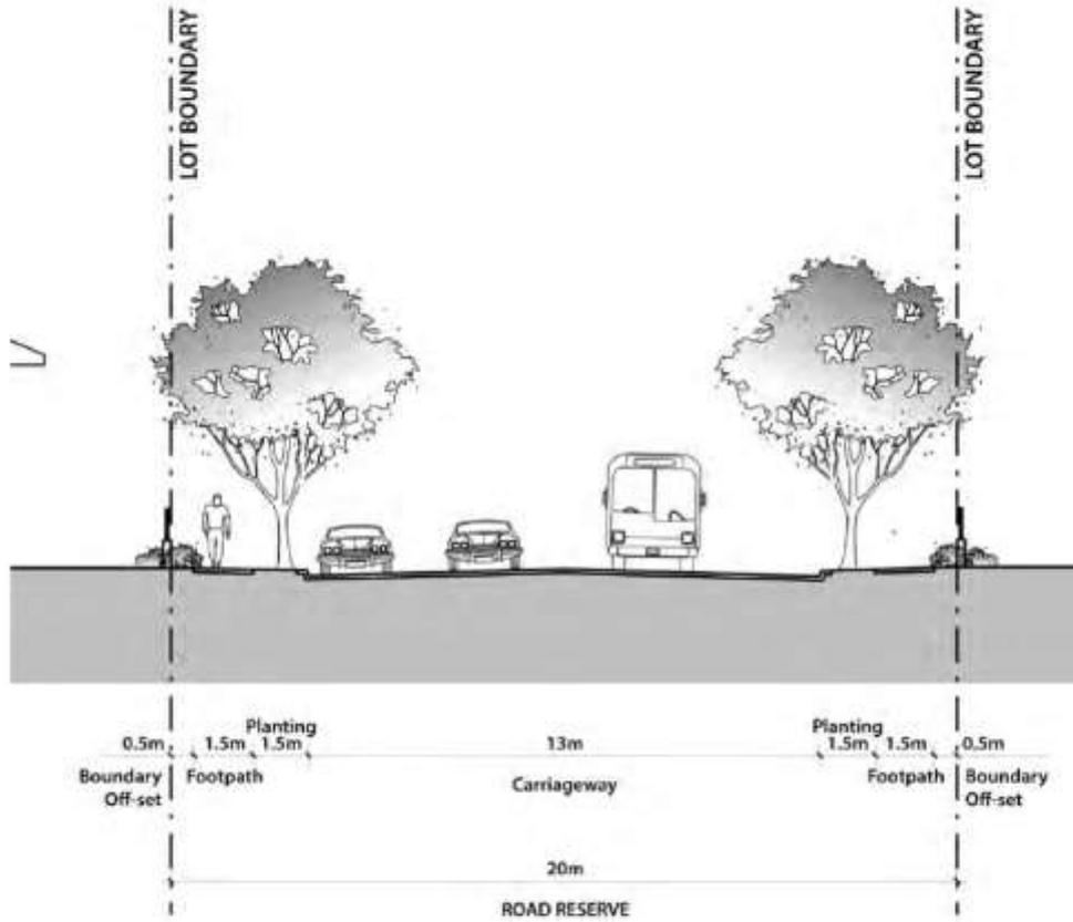
**Figure 3-13: Typical collector road (on road cycle path)**
