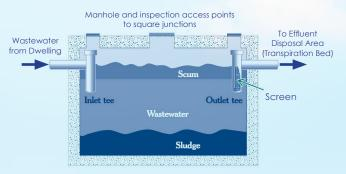
Bacteria in the septic tank break down the solid matter in the sludge and scum layers. Material that cannot be fully broken down gradually builds up in the tank and must be pumped out by a licenced contractor periodically.
