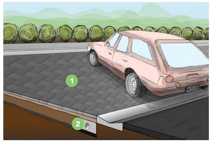
Figure 10: The functional components of permeable paving.
