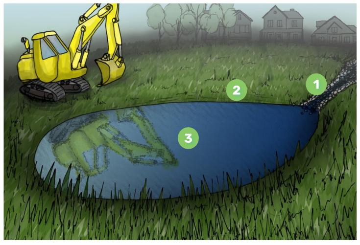
Figure 11: The functional components of a temporary sediment basin
