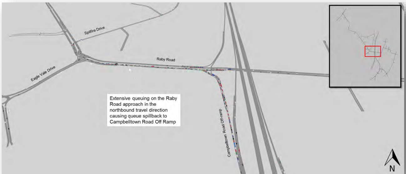
Figure 7-9 Year 2021-2026 Location 3 Deficiency (2021-2026_3_D2)
