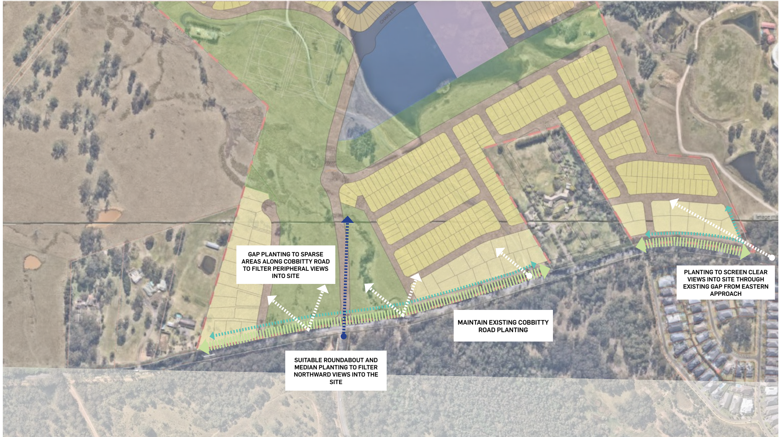
FIGURE 25 RECOMMENDED VISUAL IMPACT MITIGATION MEASURES
