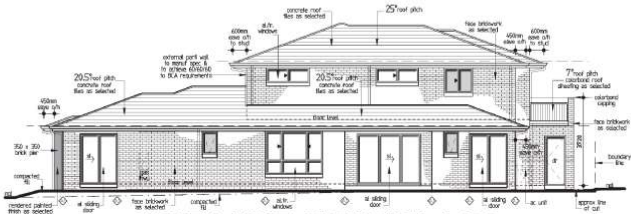
SOUTH WEST ELEVATION 1:100
