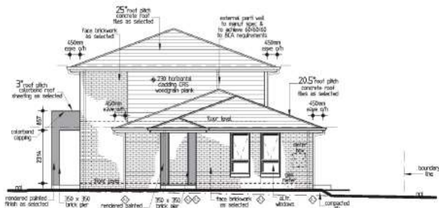
NORTH WEST ELEVATION 1:100
