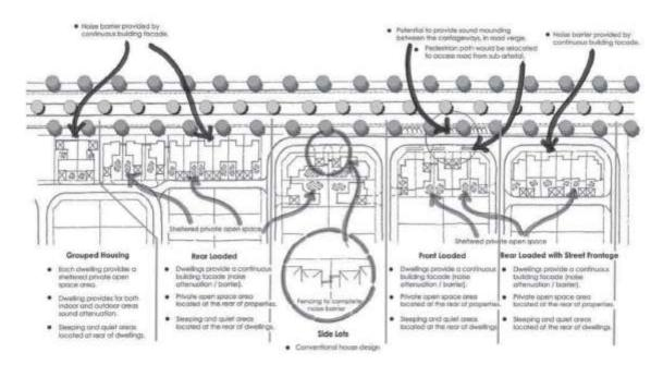
Figure 2-1 Measures to attenuate noise
