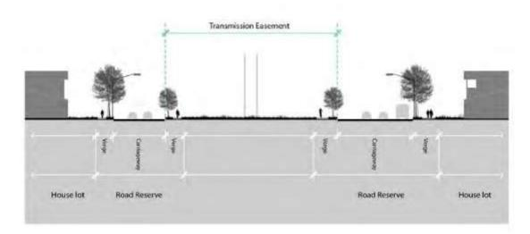
Figure 4-8: Preferred layout of development on land affected by Transmission easement
