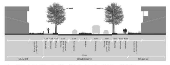
Figure 2-15: Indicative Rickard Road Transit Boulevard section (with Optional Median)
