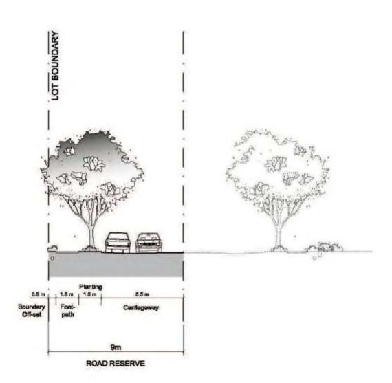
Figure 3-20 Temporary half road width construction
