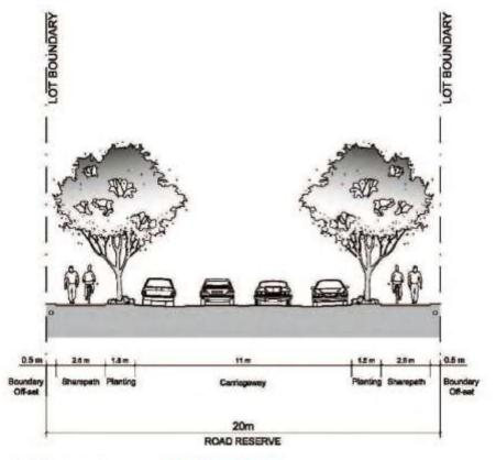
Figure 3-12: Typical collector road (off road cycle path)
