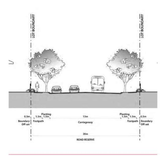
Figure 3-13: Typical collector road (on road cycle path)
