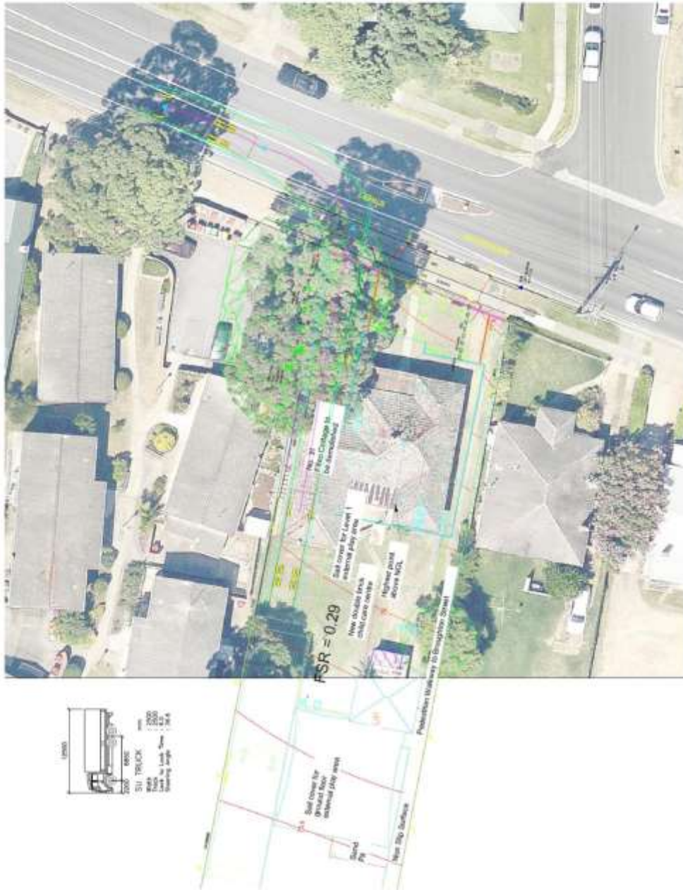
Vehicle swept path for construction vehicles – HRV (exiting the site in a forward direction)
