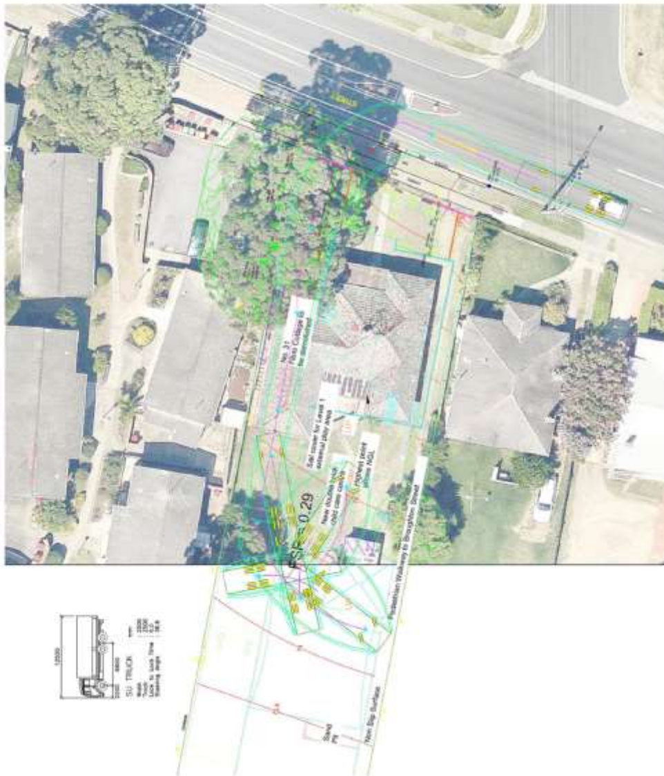
Vehicle swept path for construction vehicles – HRV (entering the site in a forward direction)
