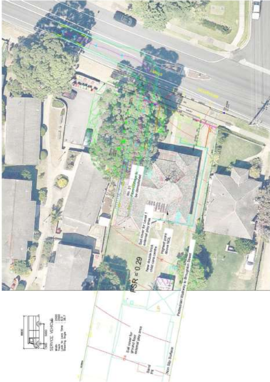
Vehicle swept path for construction vehicles – MRV (exiting the site in a forward direction)
