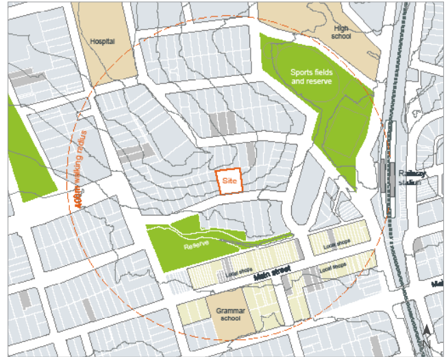
Figure 2-18 The neighbourhood scale outlines the urban grid and block structure including streets and open spaces, significant topography, heritage and civic and community uses. Proposals for individual or small groups of low rise medium density development sites should address this scale.
