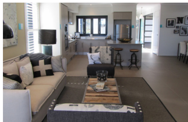
Figure 2-83 Additional floor space is required to ensure circulation can be achieved once the dwelling is furnished.
