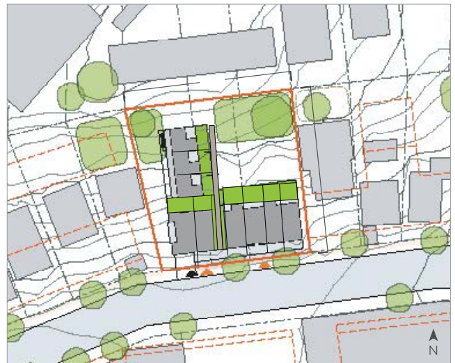
Figure 2-20 The site scale is a detailed analysis of the development's immediate context and should include the site itself, the street it addresses and surrounding properties. All proposals should address this scale.
