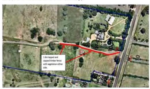
Diagram 1 - Indicative location of the proposed 1.6m high lapped and capped acoustic fence
