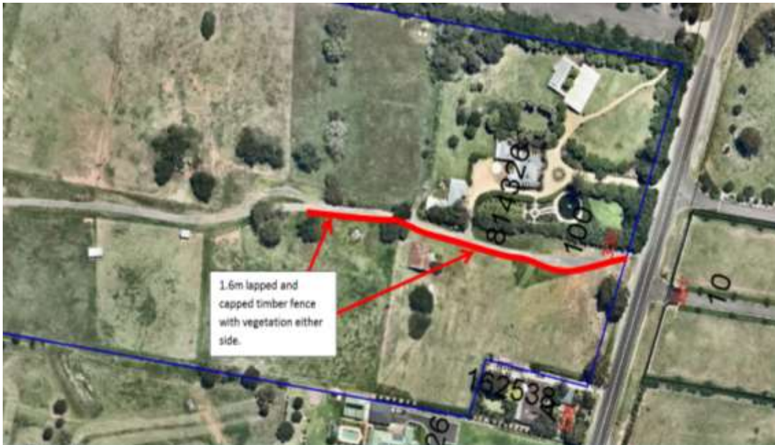
Diagram 1 - Indicative location of the proposed 1.6m high lapped and capped acoustic fence
