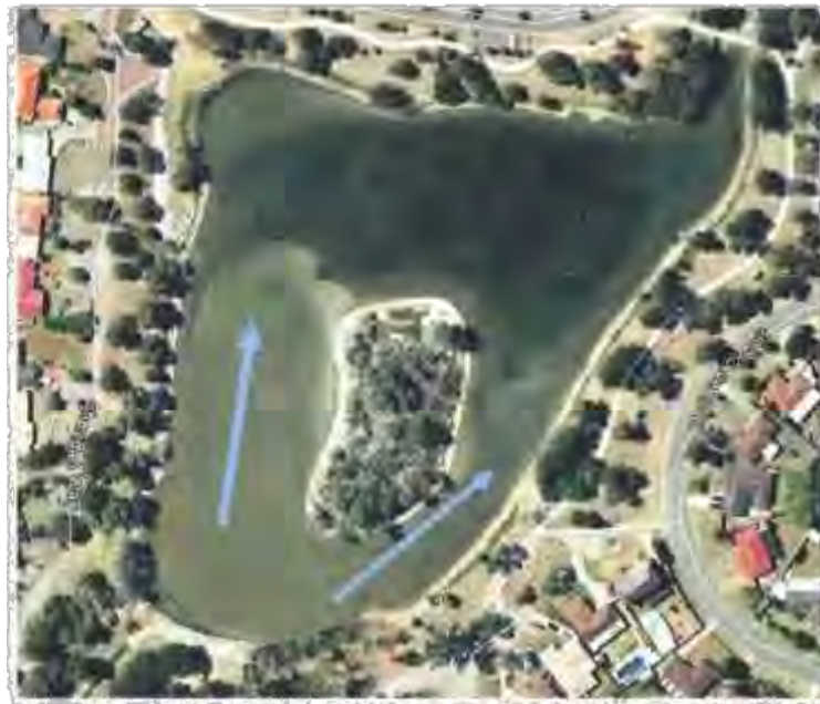
Figure 2.1 Lake inflow-sediment plume distribution behaviour. Note how sediments enter primarily from the main inflow and the flows move this sediment through the lake. Note also the presence of submerged plants in the northern section of the lake – conferring water quality improvement (this should be retained).
