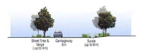
Figure C57.2 Mater Dei Local Road Section and Plan
