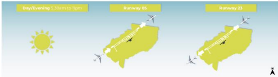
Figure 1: Proposed day/evening runway modes of operation (Source: Draft EIS: Part B – The Project (Sept 2023) p7-13)
