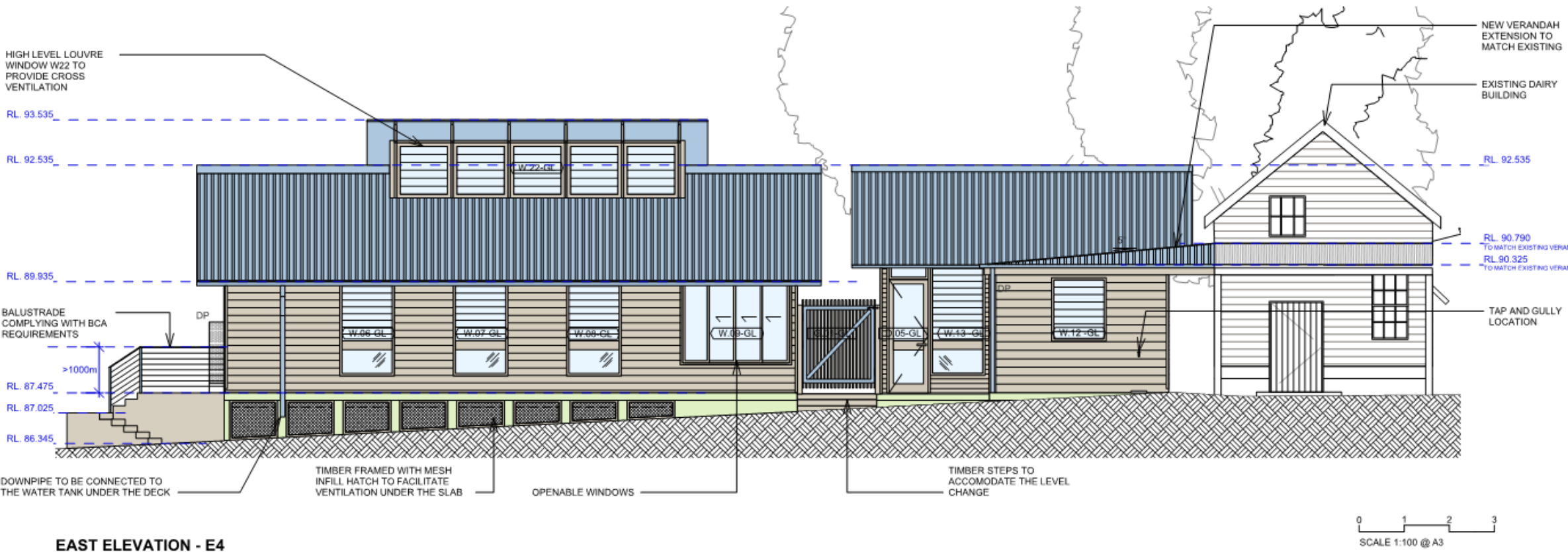
EAST ELEVATION - E4
