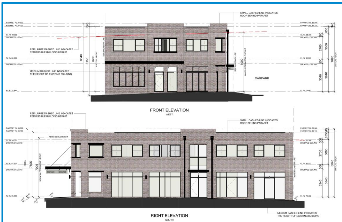
Figure 7: Extract of the elevations from the proposed plans. The dashed red line shows the 7 metres height of building limit.
